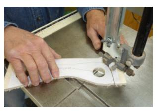
Cut out the template. First drill the 1-1/4" holes as indicated on the template. Then, use either a band saw or scroll saw to cut to the pattern lines, and sand the edges smooth.
