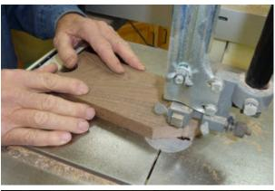
Cut rough shape on band saw. Using a band saw, cut the curved shapes, leaving the line for final shaping later.
