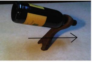
At this point it is a good idea to test the holder for balance. Before sanding, place a full 750-ml bottle of wine in the holder to see if it stays firmly balanced. You might find that it balances perfectly without further modification. If you are slightly off, it might feel 'a bit tippy'. If you are grossly off, it won't stand on its own at all. If it doesn't balance properly, carefully feel which way the holder is leaning under the weight of
